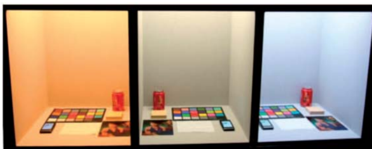
Fig. 2. The three section lighting booth
