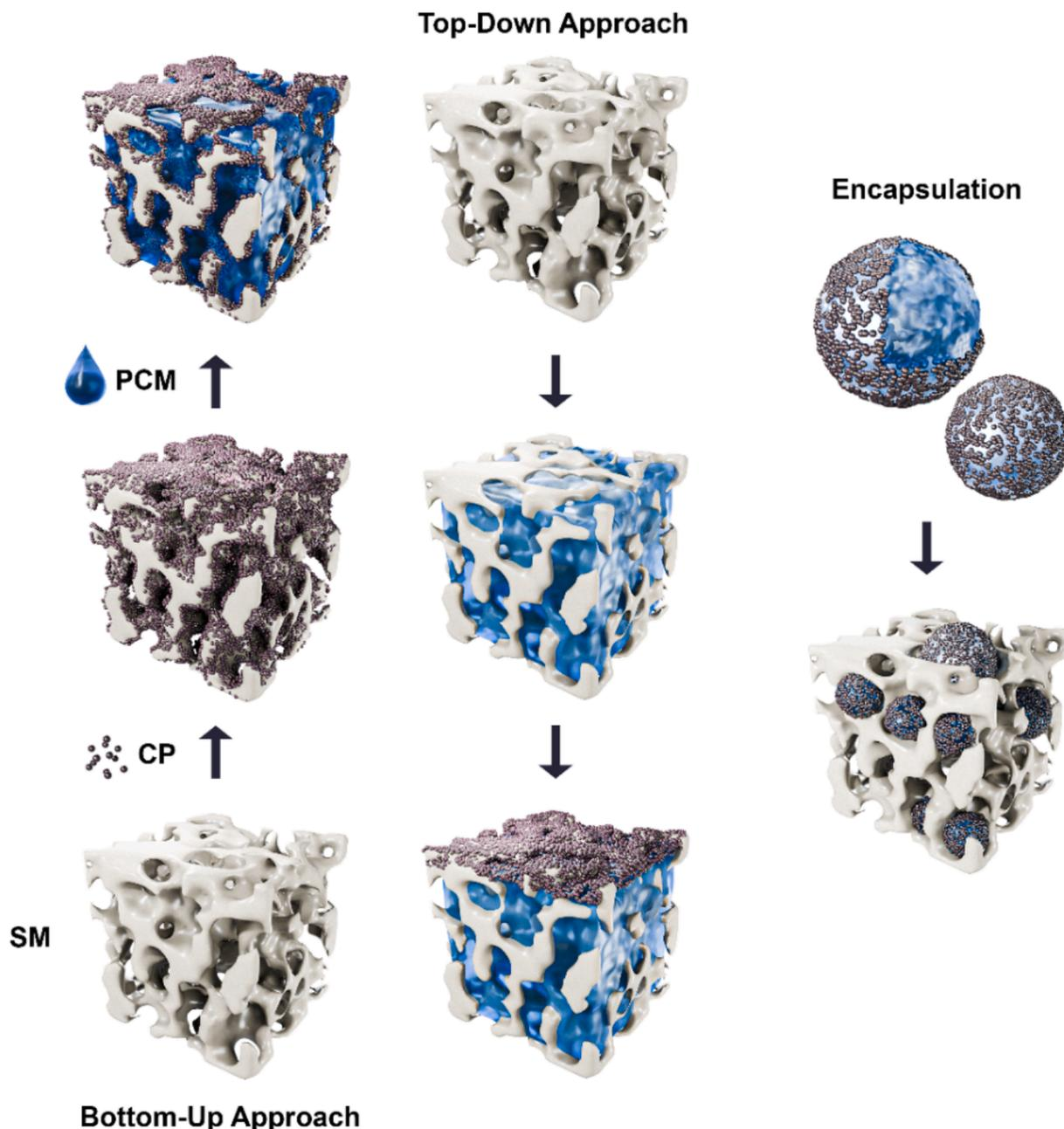
Fig. 2. The incorporation of CPs with PCMs through three distinct methods: bottom-up, top-down, and encapsulation. SM stands for the support matrix.
