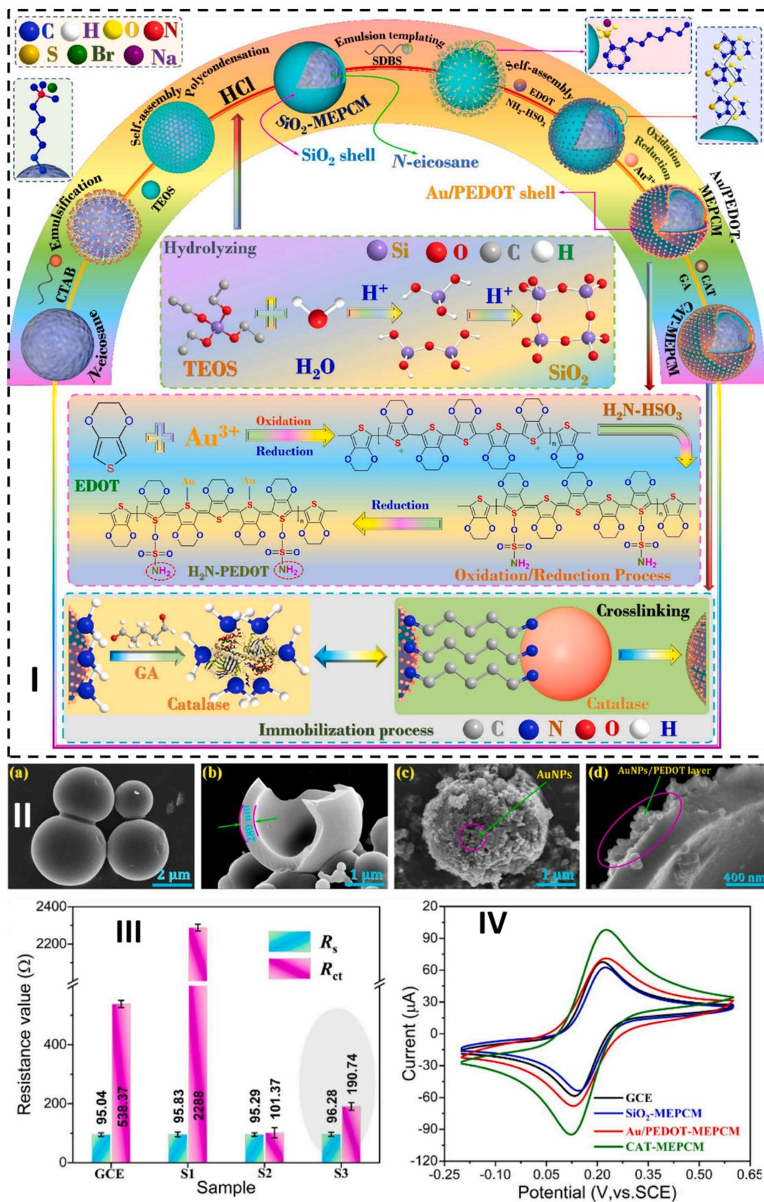
**Fig. 8.** I) Schematic presentation of preparation and reaction procedures of CAT-MEPCM. II) SEM pictures related to (a, b)  $\text{SiO}_2$ -MEPCM and (c, d) Au/PEDOT-MEPCM. III) Resistance performance related to GCE and the GCEs containing  $\text{SiO}_2$ -MEPCM (S1), Au/PEDOT-MEPCM (S2), and CAT-MEPCM (S3). IV) CV graphs of GCE and refined GCEs in the  $\text{K}_4\text{Fe}(\text{CN})_6/\text{KCl}$  electrolyte, permission from [117].
