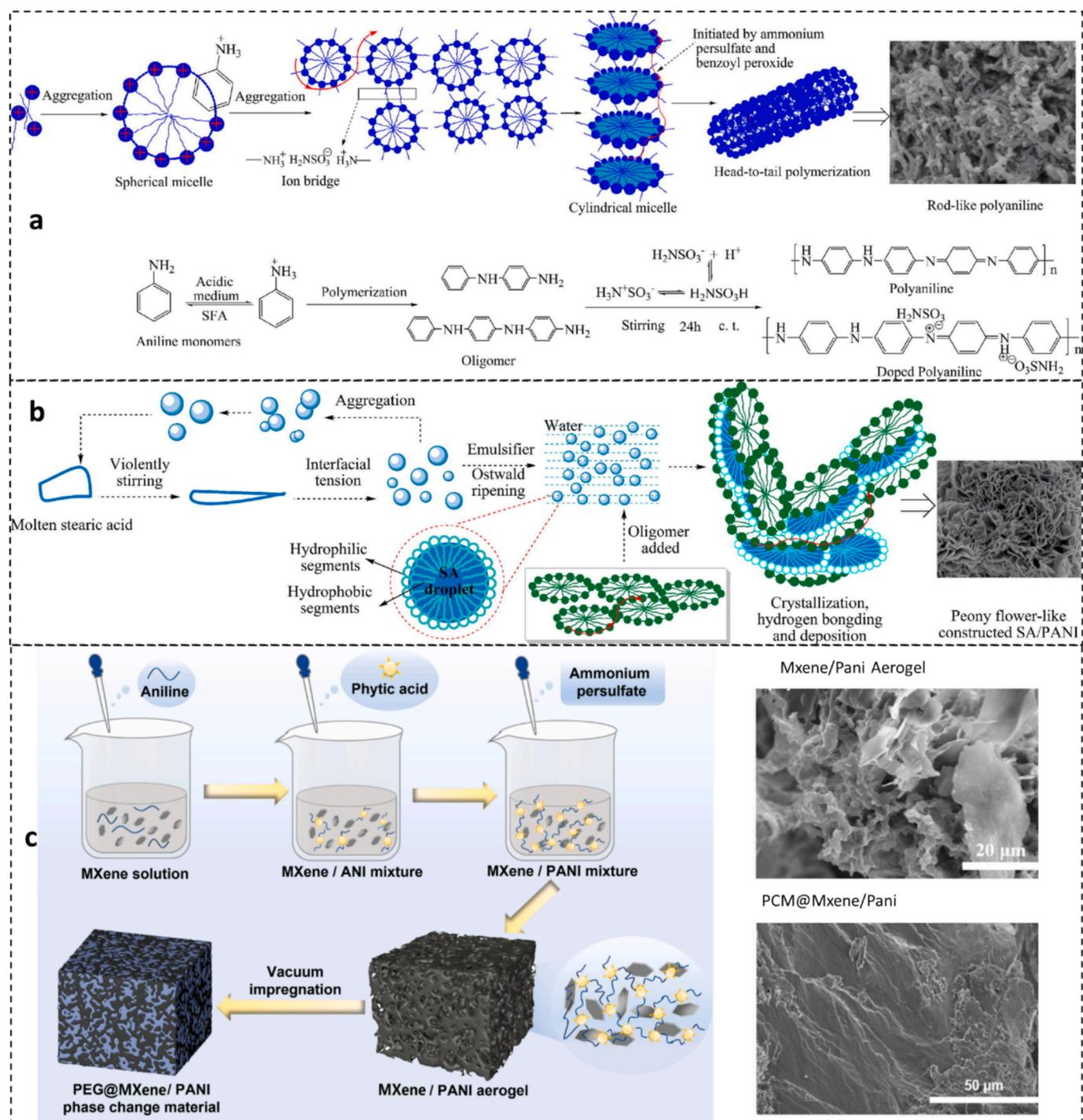
Fig. 6. A) Doping mechanism of PANi and b) the encapsulation of stearic acid with PANi, reprinting permission from [111]. c) Schematic illustration of bottom-up approach for the preparation of PEG@MXene/PANI aerogel, reprinting permission from [115].
