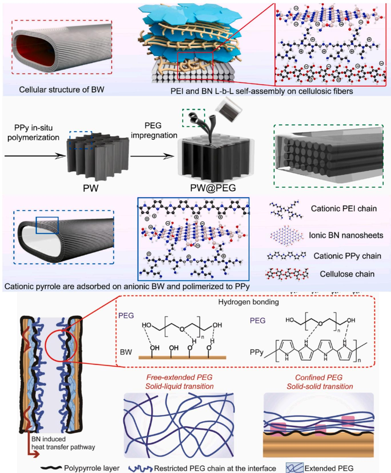
Fig. 4. Schematic illustration of bottom-up approach used for the preparation of PEG loaded PPy-wood, permission from [101].
