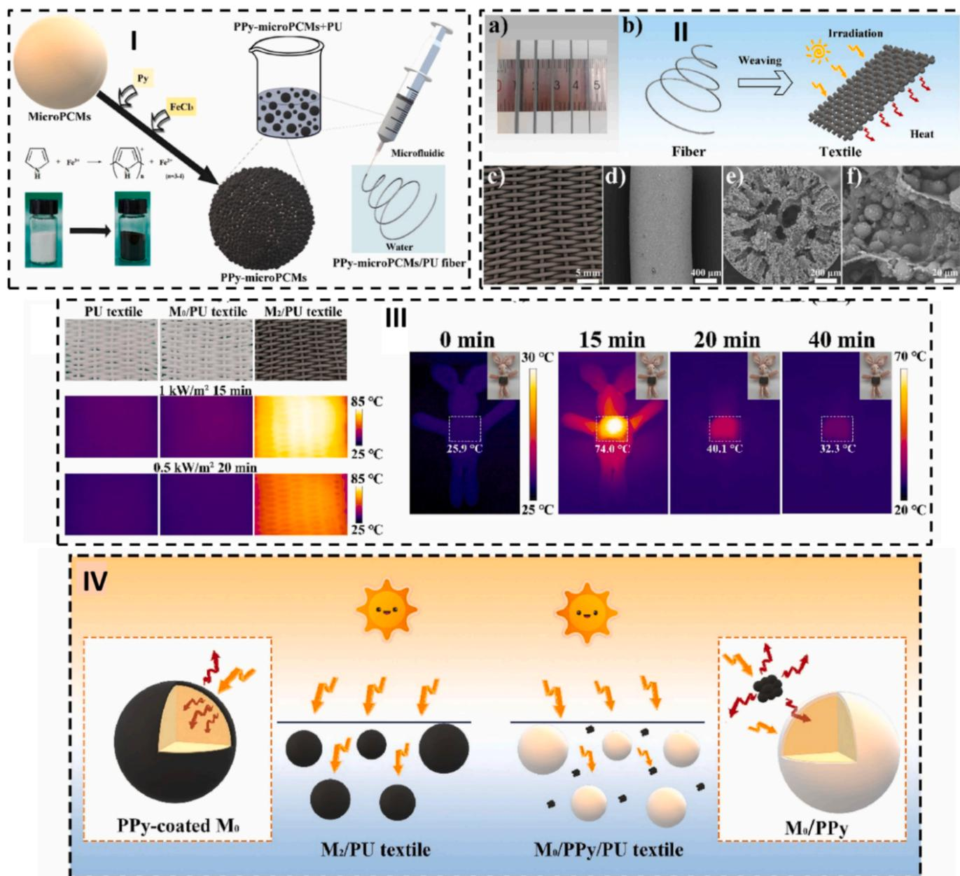
**Fig. 3.** I) The preparation route of PPy-modified PCM microcapsules-PU fibres. II) a) Image of the fibres with different thickness. b) Schematic representation of photothermal approach. c,e,f) Surface morphology of the material with different magnification. III) e) Optical and infrared images under irradiation and demonstration of thermotherapy enabled by the material. IV) Schematic presentation of photothermal efficiency, permission from [98].
