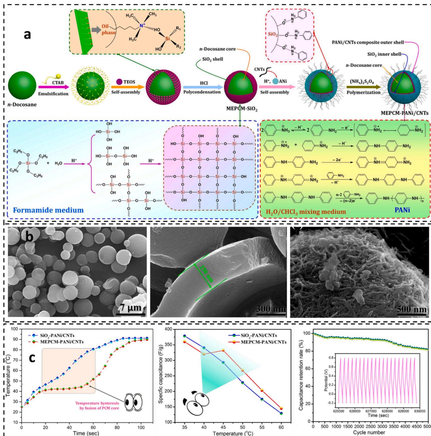
**Fig. 5.** A) Synthetic and reaction procedures for the PCM-PANI/CNTs microelectrode. B) SEM images of the microcapsules, their shell and surface structures. C) Phase change observation during heating process (left), specific capacitance versus temperature under a 1.0 A/g current density (middle), capacitance retention versus cycle number and inserted representative GCD curves at 45 °C and 2.0 A/g current density (right), permission from [113].
