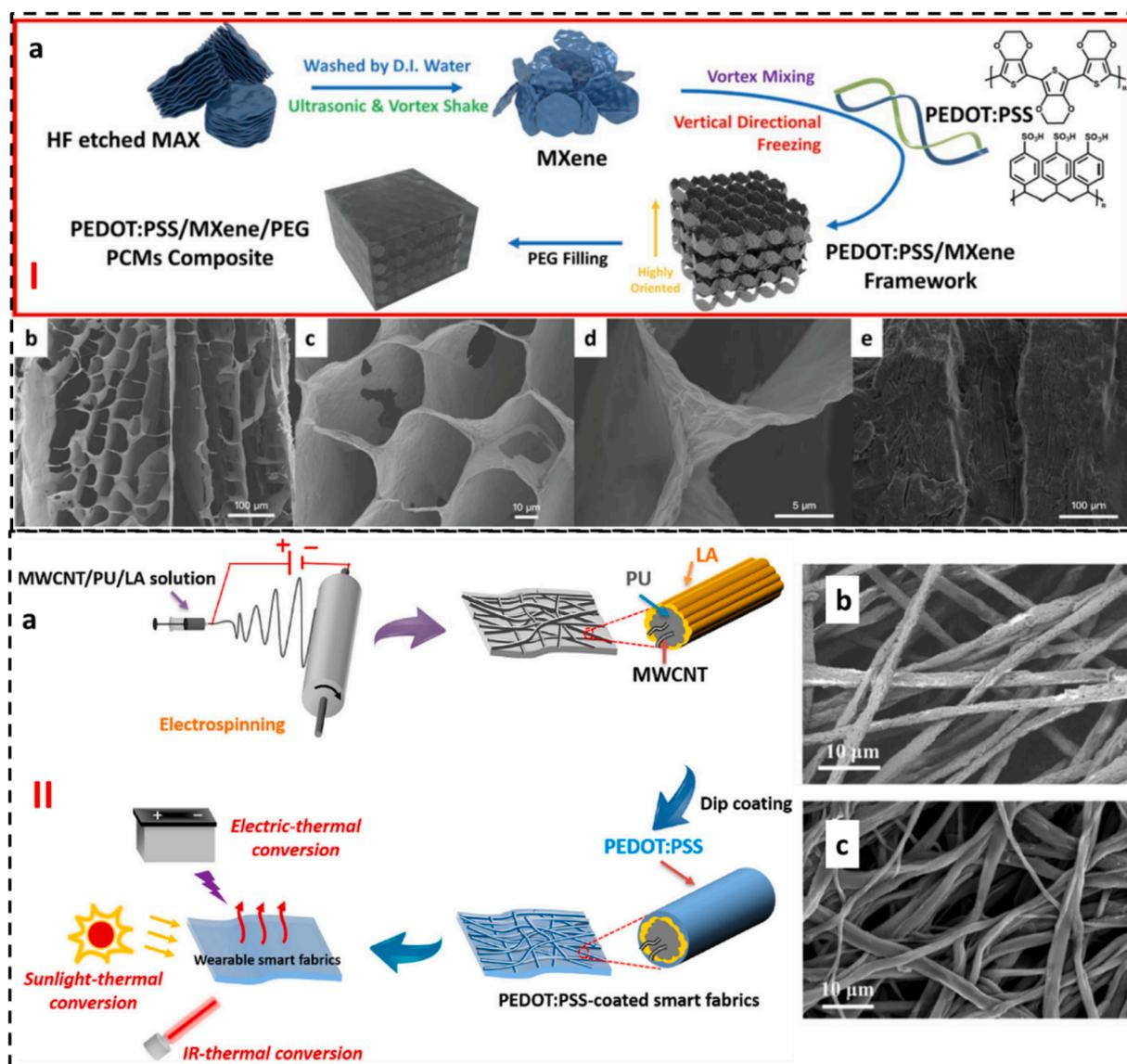
Fig. 7. I) a: Bottom-up approach used in the fabrication of PEDOT:PSS/MXene/PEG material. (b-d) SEM images of PEDOT:PSS/MXene scaffold and (e) PEDOT:PSS/MXene/PEG composite, permission from [120]. II) a: Top-down approach used in the fabrication of PEDOT:PSS-coated MWCNTs/LA/PU modified textiles and b,c) corresponding SEM images before and after coating, reprinting permission from [116].
