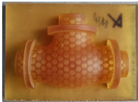
**Figure 5. 3D printed plastic pattern used in this study with a claimed thermal resistance up to 200 °C.**
