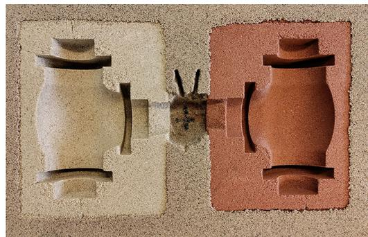
**Figure 7. Two small molds combined in a big phenolic mold (left: SSGC, right: SSFE).**
