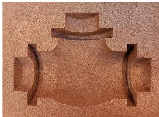
**Figure 6. One small mold prepared with solid silicate and iron(III) oxide additive(SSFE).**
