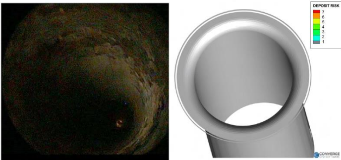
Fig. 11. OP2 deposit formation: exp (left) and sim (right)
