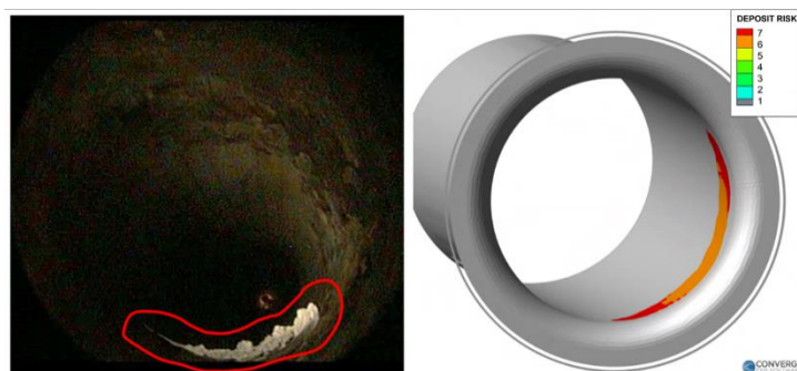
Fig. 17. OP4 deposit formation: exp (left) and sim (right)
