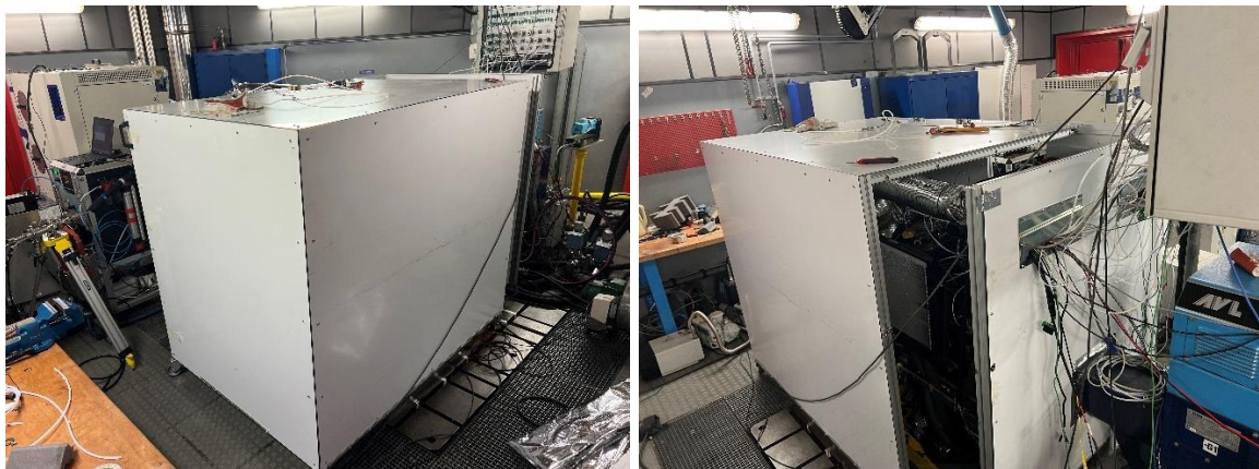
Fig. 3. Pictures of cold-box setup for -10°C engine bench tests
