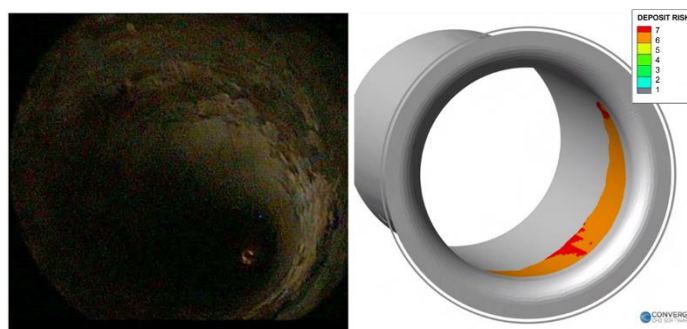
Fig. 20. OP5 deposit formation: exp (left) and sim (right)
