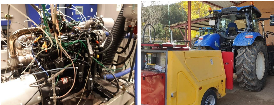
Fig. 1. Agricultural engines set in the engine test bench (left, engine w/EGR) and in the vehicle (right, engine w/o EGR)
