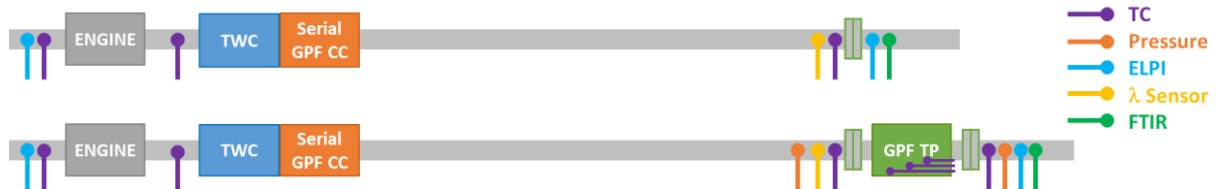
Fig. 8. Measuring points and analyzers for vehicle tests, with and without TP GPF
