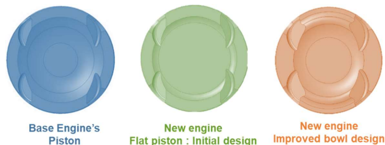
(a) Comparison of piston bowl design
