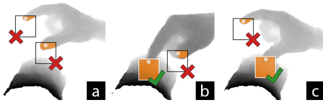
Figure 5. Touch detection. (a) When there is no touch, flood fill is restricted to filling only in parts of the finger. (b, c) When the finger touches flood fill grows into the BOH filling a larger area (White: seed point, Brown: flood filled pixels).
