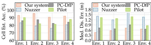
Figure 6: Comparison of cell estimation accuracy achieved by different indoor localization systems in four indoor environments
