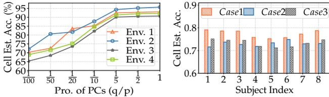
Figure 10: Cell estimation accuracy with different proportions of principle components (PCs) in four indoor environments
