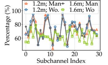
Figure 3: The probability from all the 30 subchannels that the CSI measurement changes result in destructive or constructive effect respectively when a subject blocks the LOS path in the area of interest
