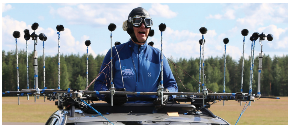
FIG. 2. (Color online) The system for measurements of the effect of flow to directional radiation from a real subject. 16 microphones and two wind speed meters surround the subject, two head-mounted microphones capture the radiated signal, and the position of the head is kept constant via a head rest. 12 m/s flow is generated by driving back and forth on a taxi road of an airport.
