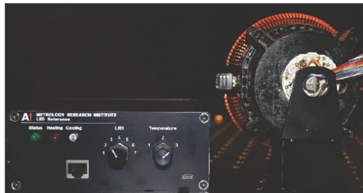
**Figure 2.** The LED based reference device comprises separate control and heat sink units.
