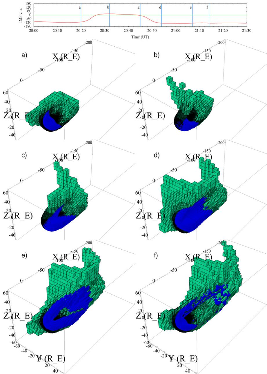
**Fig. 9.** Classification of cells in the simulation by their magnetic field topology is shown in the same format as in Fig. 8. The magnetic field topology and clock angle in the simulation are shown during and after the second AE intensification at (a) 20:20, (b) 20:32, (c) 20:45, (d) 20:54, (e) 21:07 and (f) 21:14 UT.
