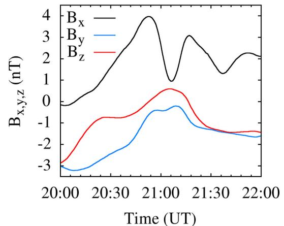
**Fig. 7.** The magnetic field observed in the simulation by a virtual satellite located at  $(-110, 5, 10) R_E$  in GSE during and after the second AE intensification.
