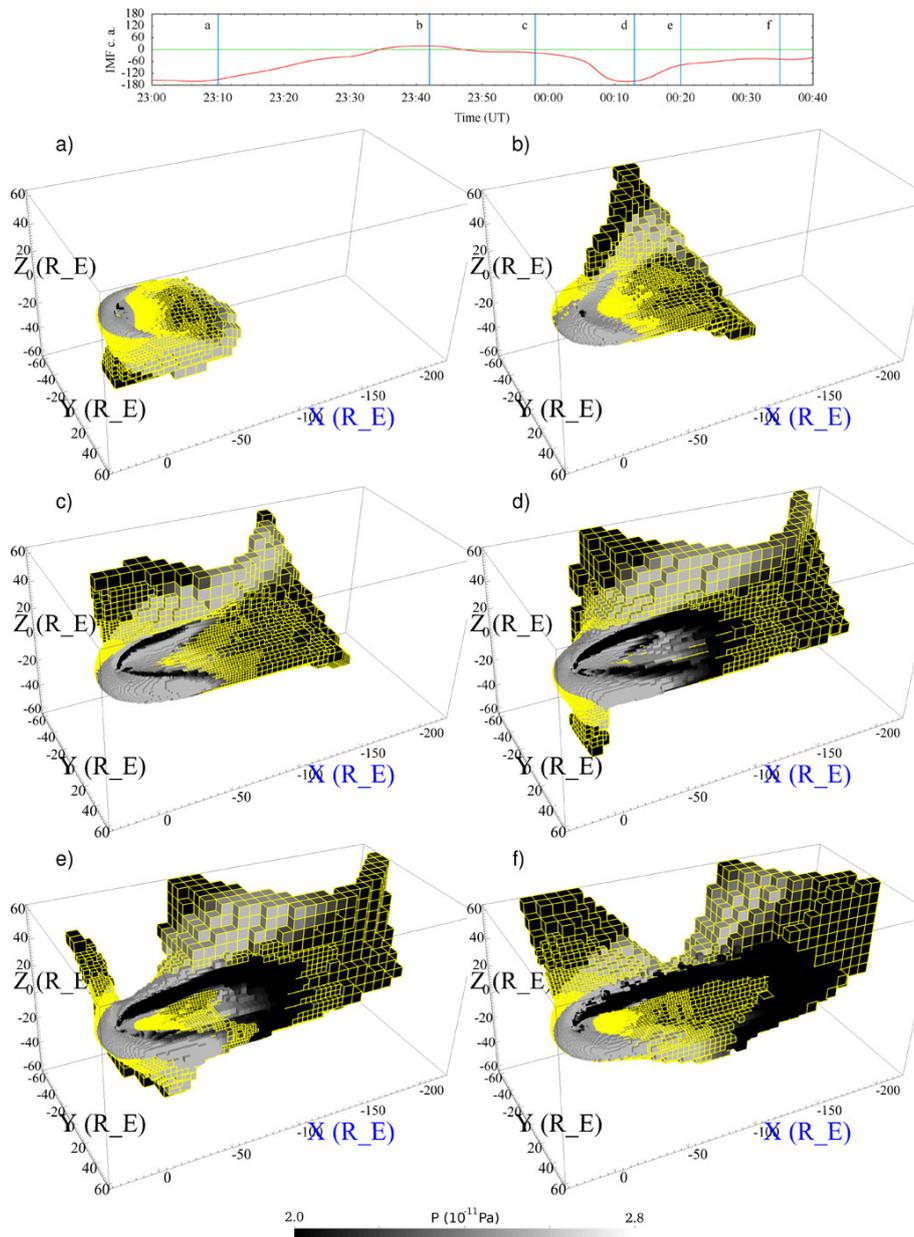
**Fig. 11.** Classification of cells in the simulation by their magnetic field topology is shown by the visible grid as in Fig. 8. Color coding shows the thermal pressure. The magnetic field topology, thermal pressure and clock angle in the simulation are shown during and after the fourth AE intensification at (a) 23:10, (b) 23:42, (c) 23:58, (d) 00:13, (e) 00:20 and (f) 00:35 UT.
