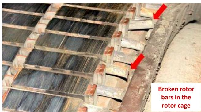
Fig.1 Example of rotor fault in a 320 kW motor operating in a mining facility.
