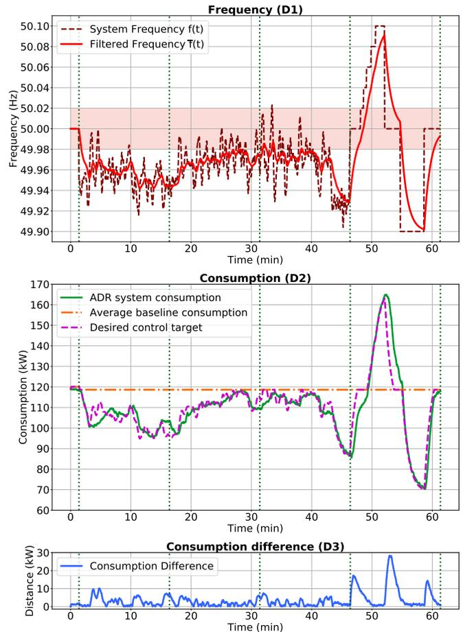
Fig. 6. (D1) The frequency  $f(t)$  injected to the ADR system using real frequency data from Fingrid [50] and custom frequency patterns, and the filtered frequency  $\bar{f}(t)$ . (D2) The realized consumption of the ADR system compared with the  $DR_{desired}(t)$ . (D3) The difference between the realized consumption of the ADR system and the  $DR_{desired}(t)$ . Moreover, the vertical dotted lines represent the time when the frequency task allocation procedure was executed by the aggregator.
