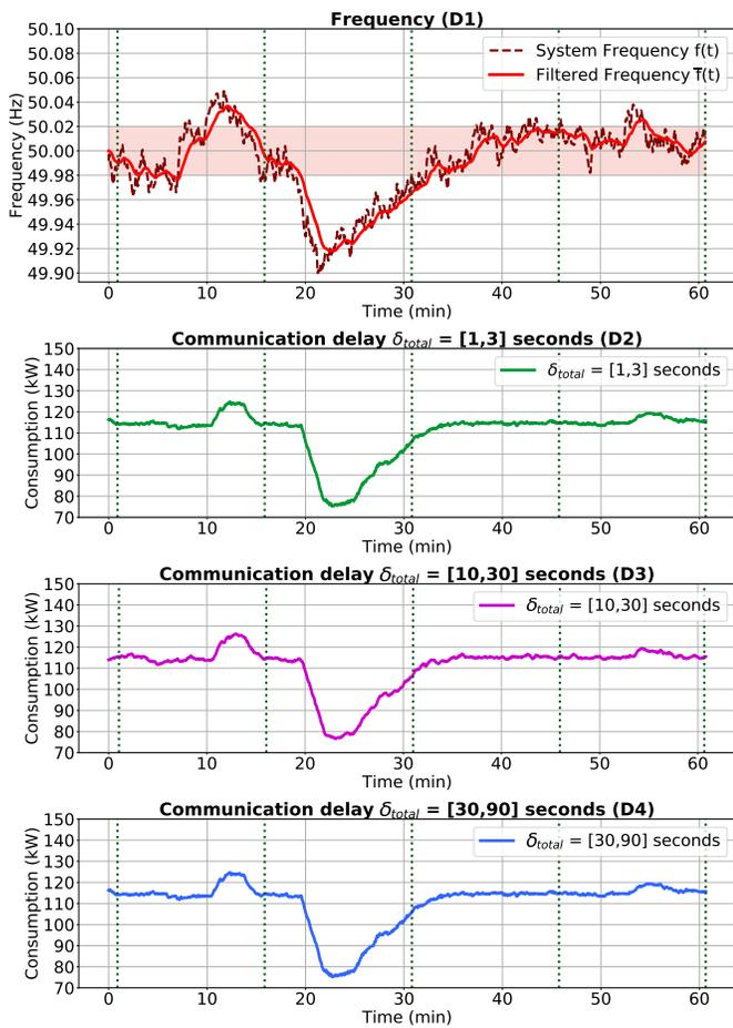
Fig. 8. (D1) The frequency  $f(t)$  injected to the ADR system using real frequency data from the Continental Europe [51]. (D2) The realized consumption of the ADR system with a  $\delta_{total}$  within the range [1,3] seconds. (D3) The realized consumption of the ADR system with a  $\delta_{total}$  within the range [10,30] seconds. (D4) The realized consumption of the ADR system with a  $\delta_{total}$  in the range [30,90] seconds.
