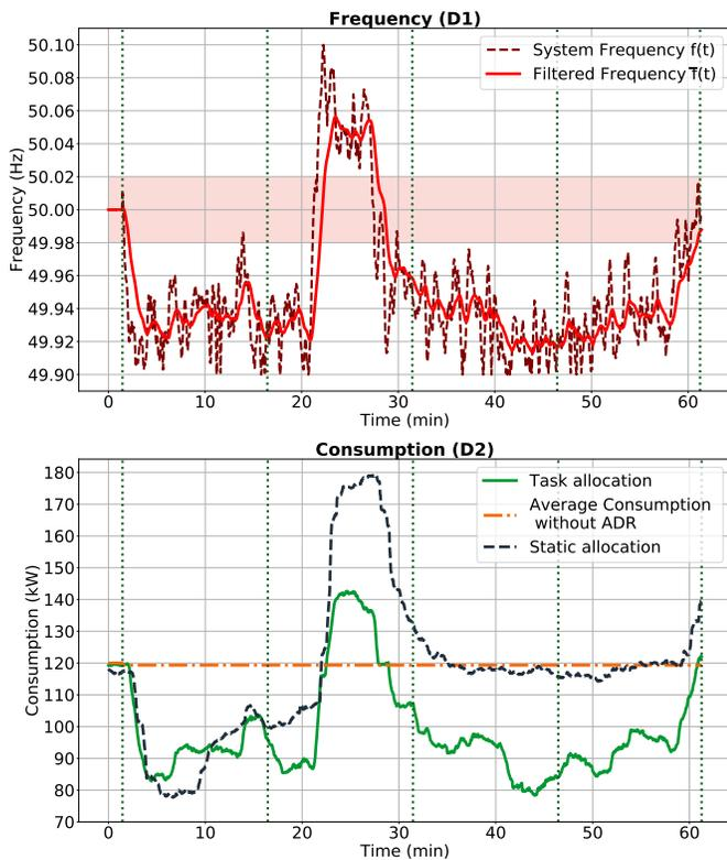
Fig. 10. (D1) The frequency  $f(t)$  injected to the ADR system using real frequency data from Fingrid [50], and the filtered frequency  $\bar{f}(t)$ . (D2) The comparison of the provided reserve of the ADR system based on the task allocation with the static allocation of energy resources presented in [11].
