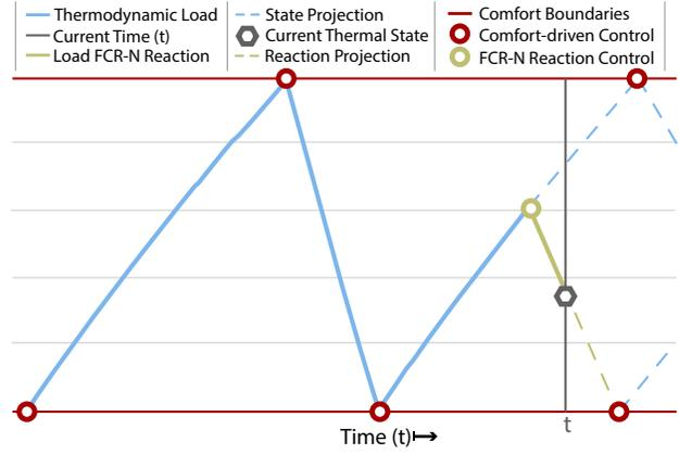
Fig. 5. Example of the control applied to a thermodynamic energy resource in order to provide FCR-N reserves while maintaining the comfort constraints.
