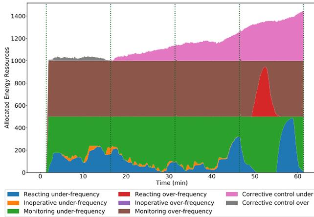
Fig. 7. The energy resources allocated to the *Allocated* composite state over time for the under-frequency and the over-frequency cases, and the amount of energy resources used by the corrective control in one hour simulation.
