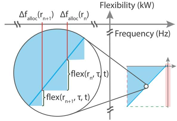
Fig. 4. The allocation of the energy resources performed by the frequency task allocation procedure. The flexibility  $flex(r_{next}, \tau_1, t)$  of the *Available* energy resources are collected in sequence and each resource is allocated with a reaction policy that specifies the respective frequency deviation  $\Delta f_{alloc}(r_{next})$ .
