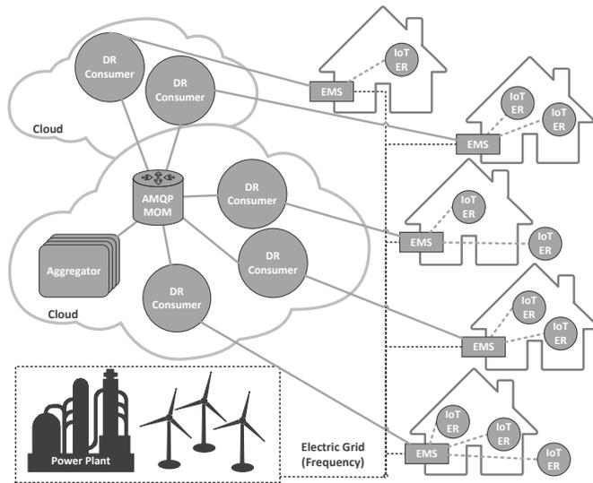
Fig. 1. An overview of the ADR system for frequency control.
