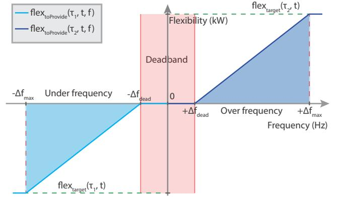
Fig. 2. The objective function  $flex_{toProvide}(\tau, t, f)$  and the target reserve function  $flex_{target}(\tau, t)$  for both the under-frequency and the over-frequency tasks.
