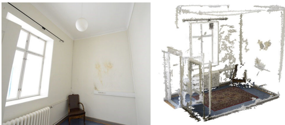
FIG. 1. Segment of an example image from an individual room (left). The white walls proved to be too featureless for image matching (right).
