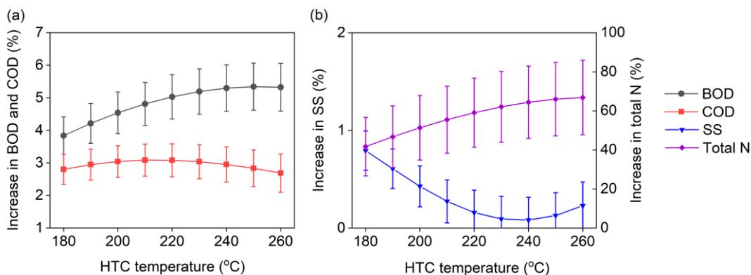
Fig. 3: Estimated increase in (a) BOD and COD and (b) suspended solids (SS) and total nitrogen loads to the wastewater treatment plant with recycling of the HTC filtrate. Error bars denote the 95% confidence intervals of prediction based on the respective regression models. Uncertainties related to the dry solids content of separated char and mass yields of the filtrate were neglected.
