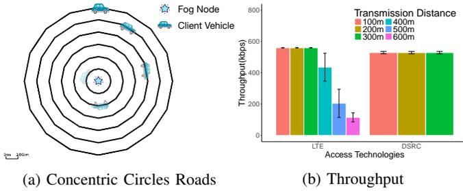
Fig. 4: Network performance of LTE vs. DSRC
