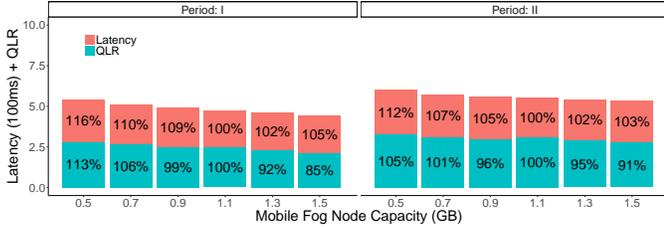
Fig. 8: Performance vs. Memory Capacity
