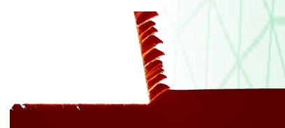
Figure 5. High resolution SPH simulation results of 2D orthogonal cutting with 500'000 particles computed on GPU.
