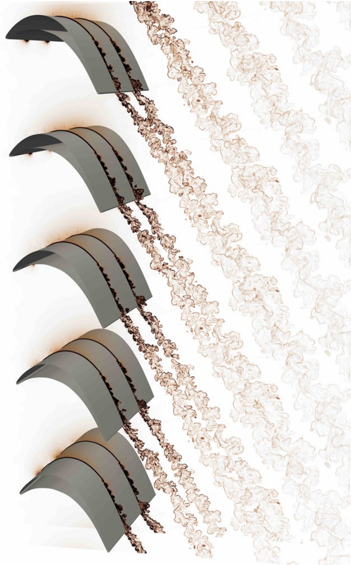
Figure 4. Flow over a T106D low-pressure turbine linear cascade [11] (copyright Vincent et al. reused with permission).
