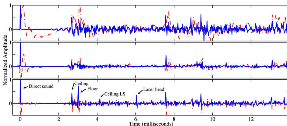
Fig. 3. (Color online) Measured (dashed-dotted line) and deconvolved (solid line) room impulse responses for spherical loudspeaker (upper box), directional loud-speaker (middle box) and LIB (lower box).
