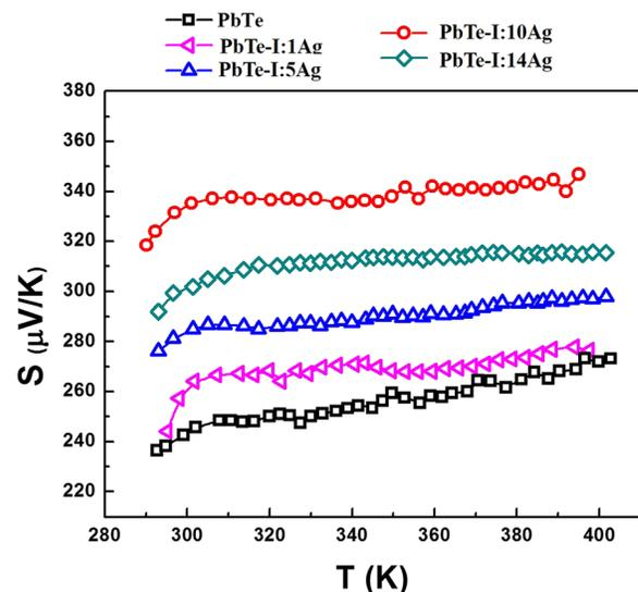
FIG. 15. Thermoelectric powers of PbTe, PbTe-I:1Ag, PbTe-I:5Ag, PbTe-I:10Ag, and PbTe-I:14Ag thin films in the temperature range of 300 K–400 K.
