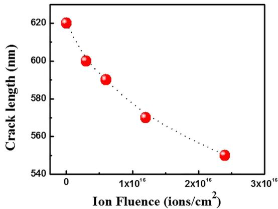
FIG. 13. Variation of crack length with ion fluence.
