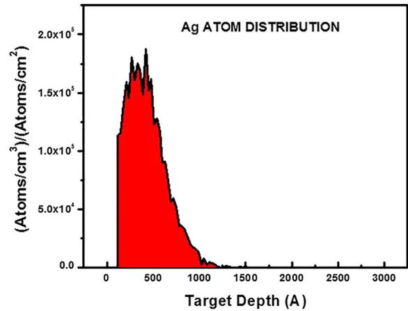
FIG. 3. TRIM simulation for atomic distribution of Ag in implanted PbTe.
