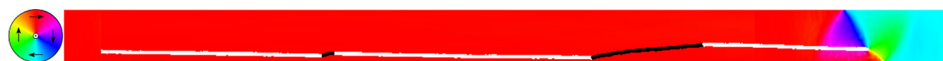
FIG. 8. The trajectory of a vortex wall moving through a polycrystalline Permalloy nanowire, 400 nm wide and 10 nm thick. The core is driven by a current density of 17 \times 10^{12} \text{ A/m}^2 which is larger than the Walker breakdown. The exchange coupling at the grain boundaries is reduced to 40% of its original value. The white/black colors indicate a positive/negative vortex core polarization. The core switches its polarization at a grain boundary and consequently changes its transverse propagation direction. As a result, the vortex core stays in the body of the nanowire and the domain wall never transforms into a transverse wall.
