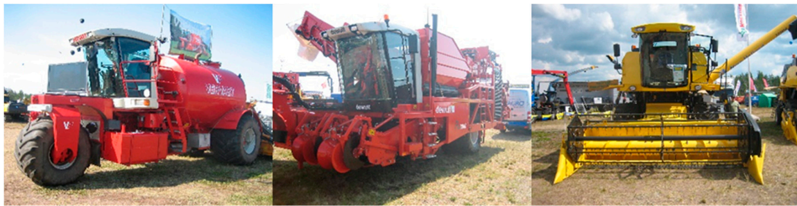
Figure 1. Examples of self-propelled agricultural machinery: Vervaet slurry spreader, Dewulf potato harvester, and New Holland TC5050 combine harvester (Photos: Antti Lajunen).
