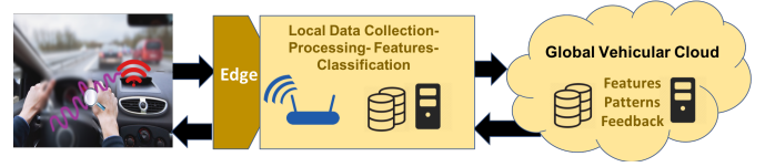
Fig. 4: Depiction of end to end WiBot computation and latency at edge and extension to cloud.
