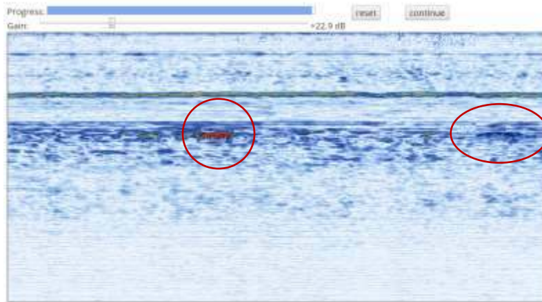
Figure 4. Shape of the flaw can be distinguished even though amplitude response is close to noise
