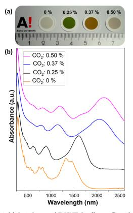
Figure 1. (a) Optical image of SWCNT thin films on filters obtained from different  $CO_2$  concentration at 850 °C and (b) corresponding absorption spectra.
