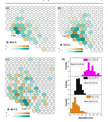
**Figure 3.** Chirality distribution of individual SWCNTs with  $CO_2$  concentration of (a) 0 vol %, (b) 0.25 vol %, and (c) 0.50 vol % at 850 °C. The insets represent the number of metallic and semiconducting tubes. (d) Diameter distribution of individual SWCNTs summarized from (n,m) maps with different  $CO_2$  concentration.
