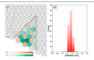
Figure 4. (a) Chirality and (b) diameter distribution of SWCNTs with 0.25 vol % CO<sub>2</sub> at 880 °C.
