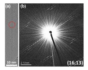
Figure 2. (a) Typical TEM image of an individual SWCNT and (b) its corresponding electron diffraction pattern with  $CO_2$  concentration of 0.50 vol % at 850 °C.
