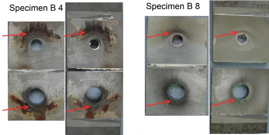
Figure 11. Specimens B 4 and B 8 after fatigue loading and disassembly.
