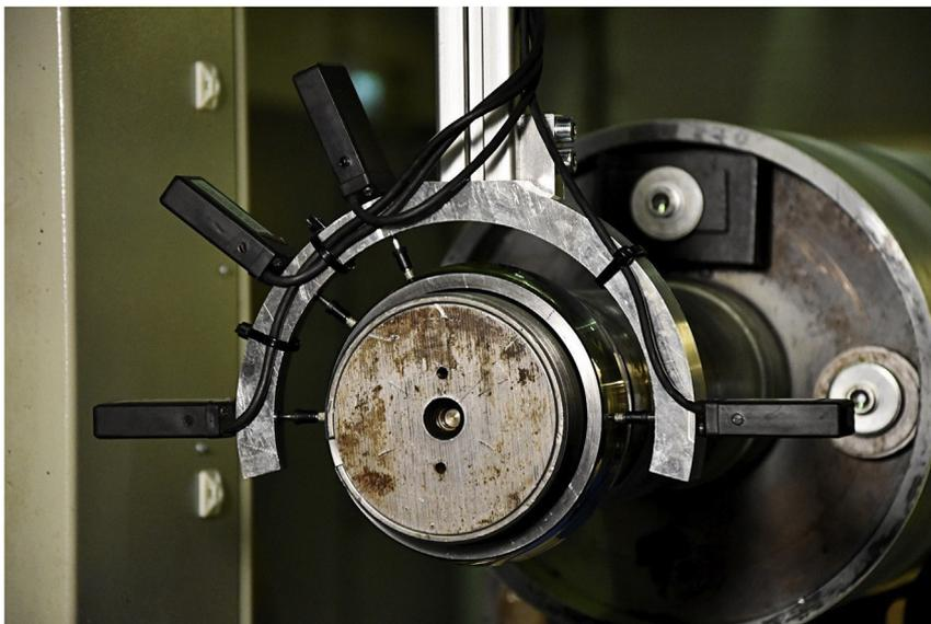
Fig. 4. Bearing inner ring measurement setup. The bearing inner ring was measured, while installed on the rotor shaft. Other bearing components, such as roller elements, roller element holders and outer ring were uninstalled prior to the measurement. During the measurement, the rotor was supported with two additional rollers.
