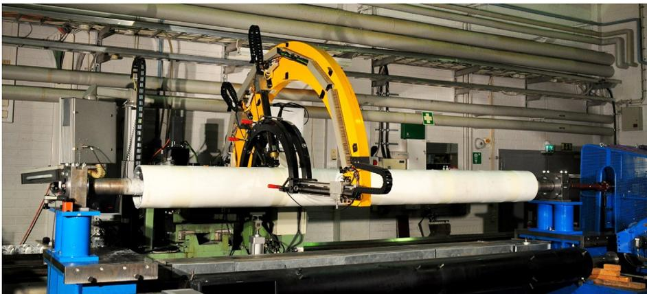
Fig. 1. Rotor dynamic response measurement setup built on a roll grinding machine.
