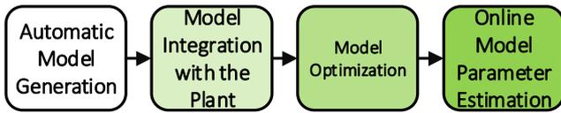
Fig. 3. Proposed method for automatic generation of SBDT.
