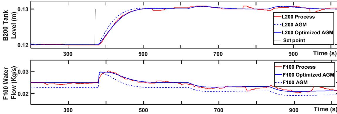
Fig. 7. Comparison of the automatically generated model (AGM) results before and after its optimization using the simulation architecture presented in [9].
