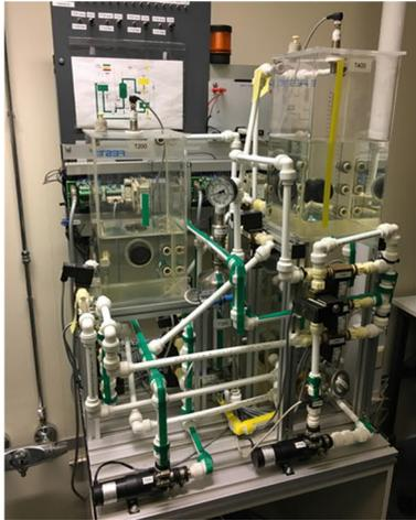
Fig. 4. Heat production plant used as a testbed of the proposed method
