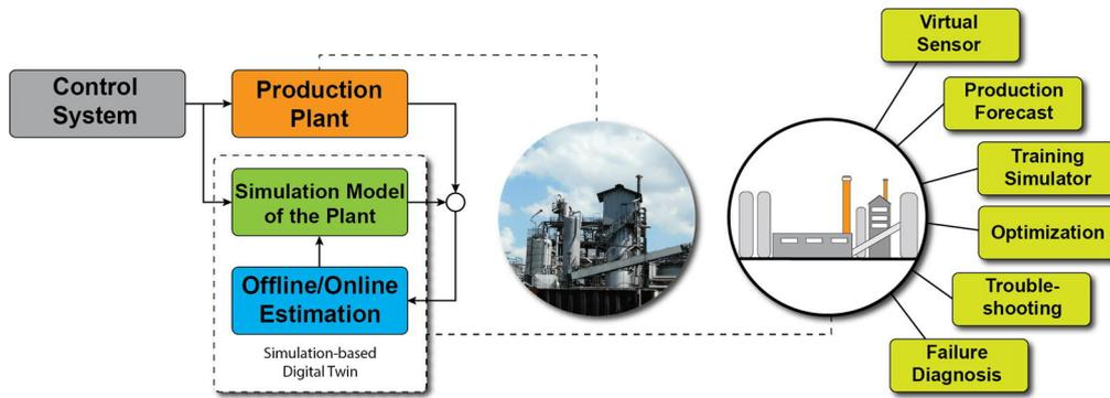
Fig. 1. Simulation-based digital twin and its applications during the operation and maintenance phases of the plant lifecycle. *Virtual Sensor* refers to the application in which non-measured information of the current state of the process can be derived from the underlying FPM of the SBDT.
