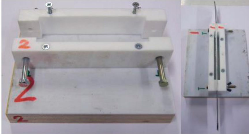
FIGURE 3: Formwork setup of fabric-reinforced test specimen.
