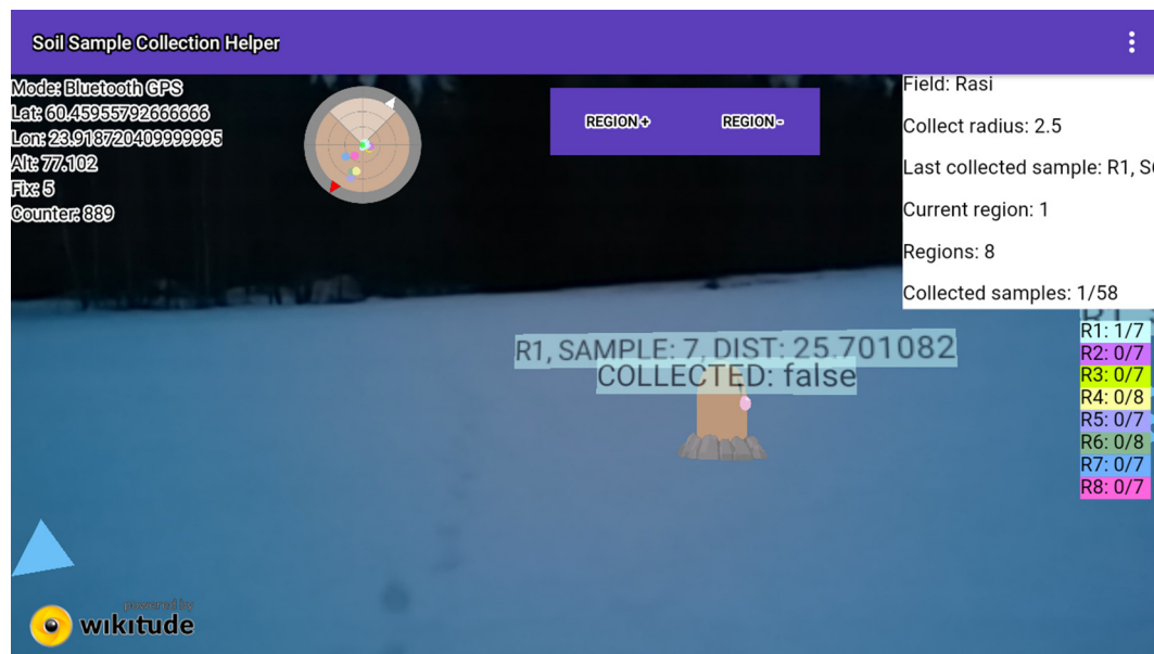
Fig. 5. View seen through the AR smartglasses. A sample point in an active region is shown.
