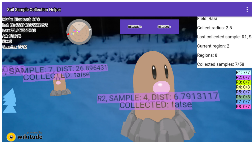
Fig. 15. View seen through the AR smartglasses. The distance to the locations indicated by the virtual marks does not match how they are perceived in the view.
