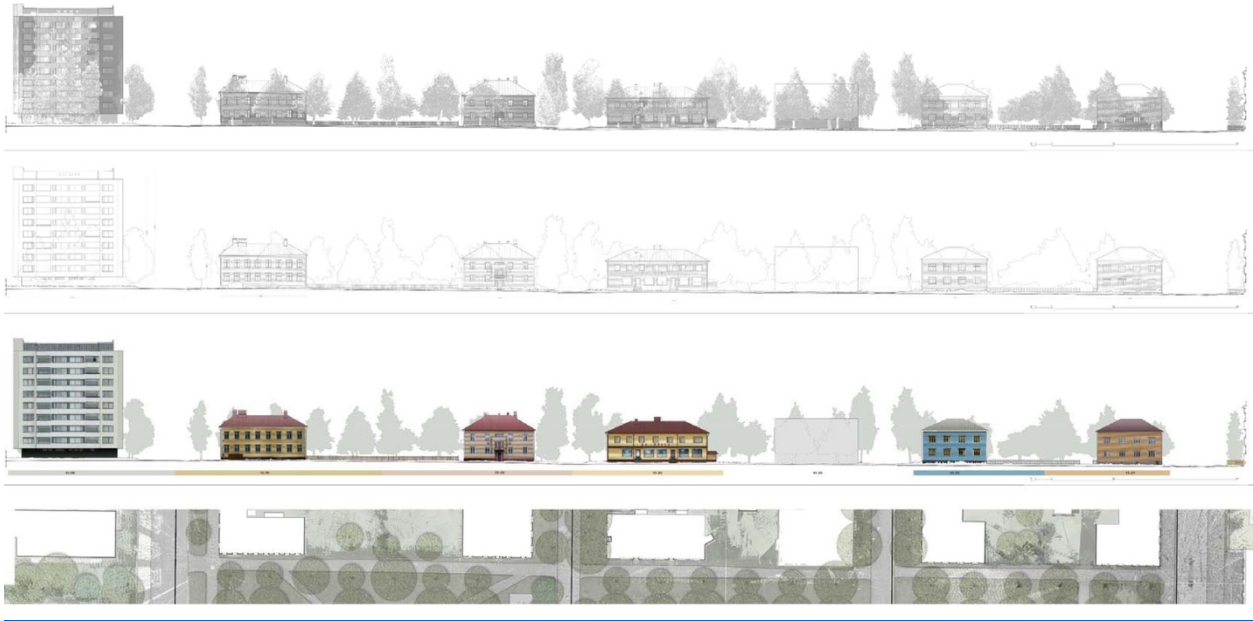
Fig 8. Description of one street front of Raksila neighbourhood. CAD drawings allow the check of measurements. Photomaps define the real image of the place and give information on colors. The map redrawn from the point cloud has been enriched with the description of the system of trees, paths and roads with identification of different materials.
