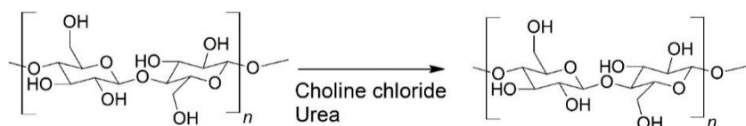
Figure 2. Non-derivative pre-treatment of cellulose with urea-choline chloride DES.
