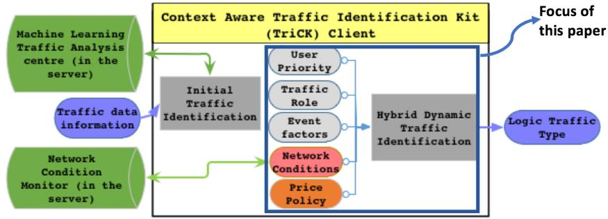
Fig. 1. Cognitive Traffic Identification Kit in Client
