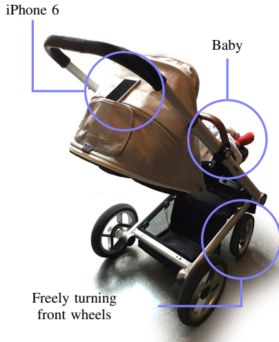
Fig. 3. The experiment setup with a wheeled baby pushchair/stroller and an iPhone placed on the top for tracking.
