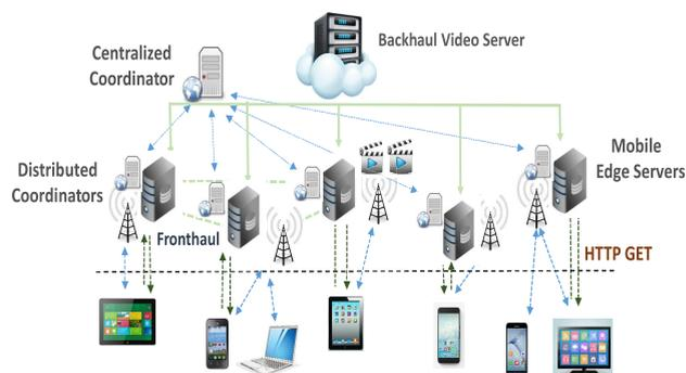
FIGURE 1. Collaborative caching at the network edges.
