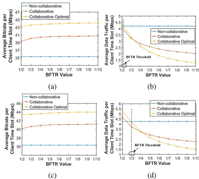
**FIGURE 7.** Impact of BFTR parameter on (a) Average video bitrate and (b) Average data traffic for different arrival intervals and (c) Average video bitrate and (d) Average data traffic for different retention curves.
