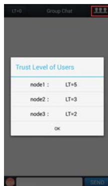
FIGURE 14. Trust level of other nodes evaluated by a local device.
