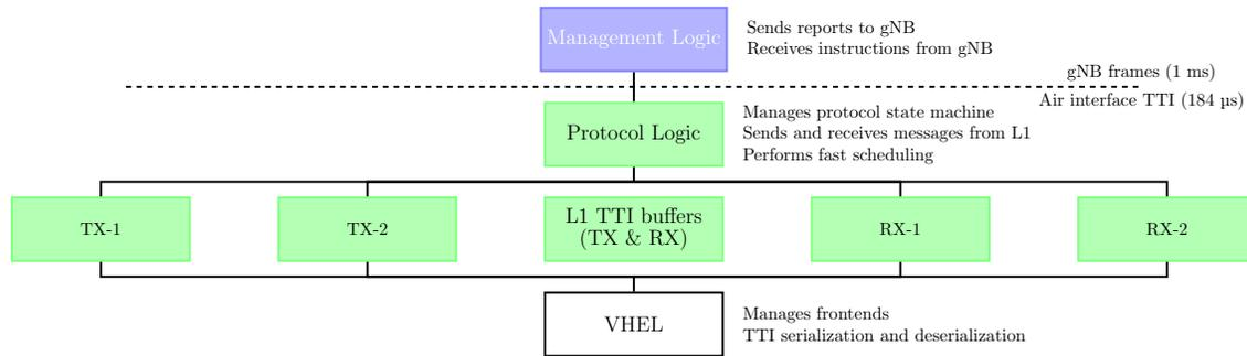
Fig. 2. Main components of the ARF software architecture.
