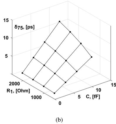
Fig. 4. (a) Implemented delay cell layout; (b) code 7 and code 5 delays difference  $\delta_{75}$  for changing  $R_1$ ,  $C$  values in the model.
