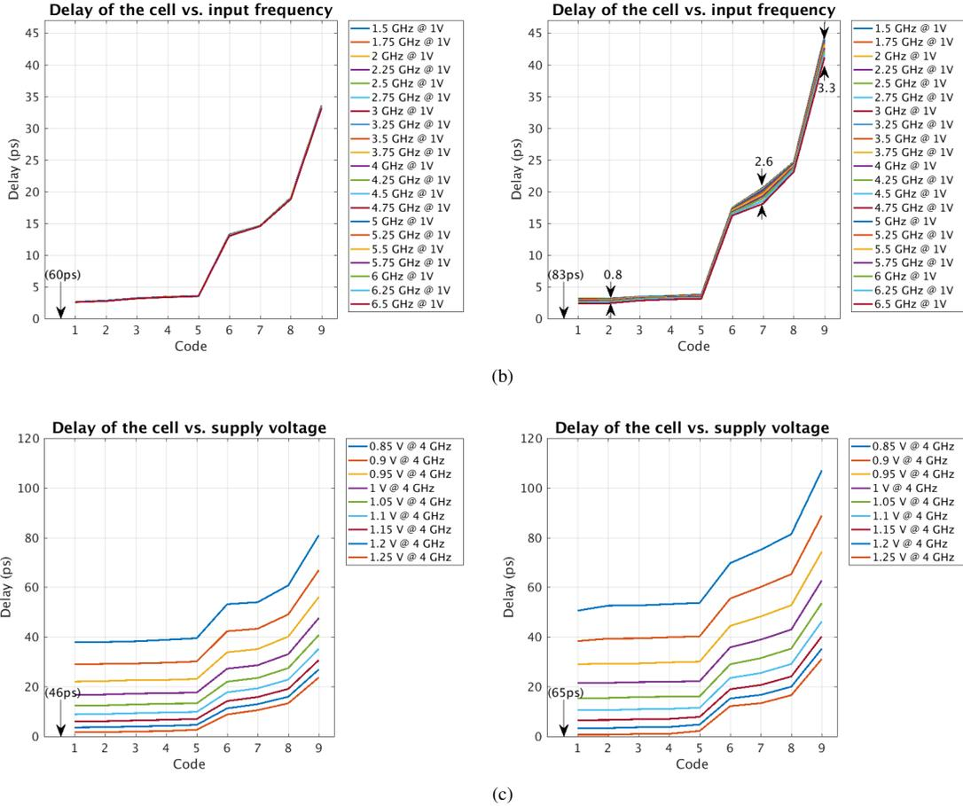
Fig. 3. (a) Simulation testbench with exercised codes and (b)-(c) simulation results for the cell circuit with physical device models (left column) and cell layout with RC-extracted parasitics (right column). Shown in parenthesis is the smallest intrinsic delay of the cell; bounded with arrows is the delay spread.
