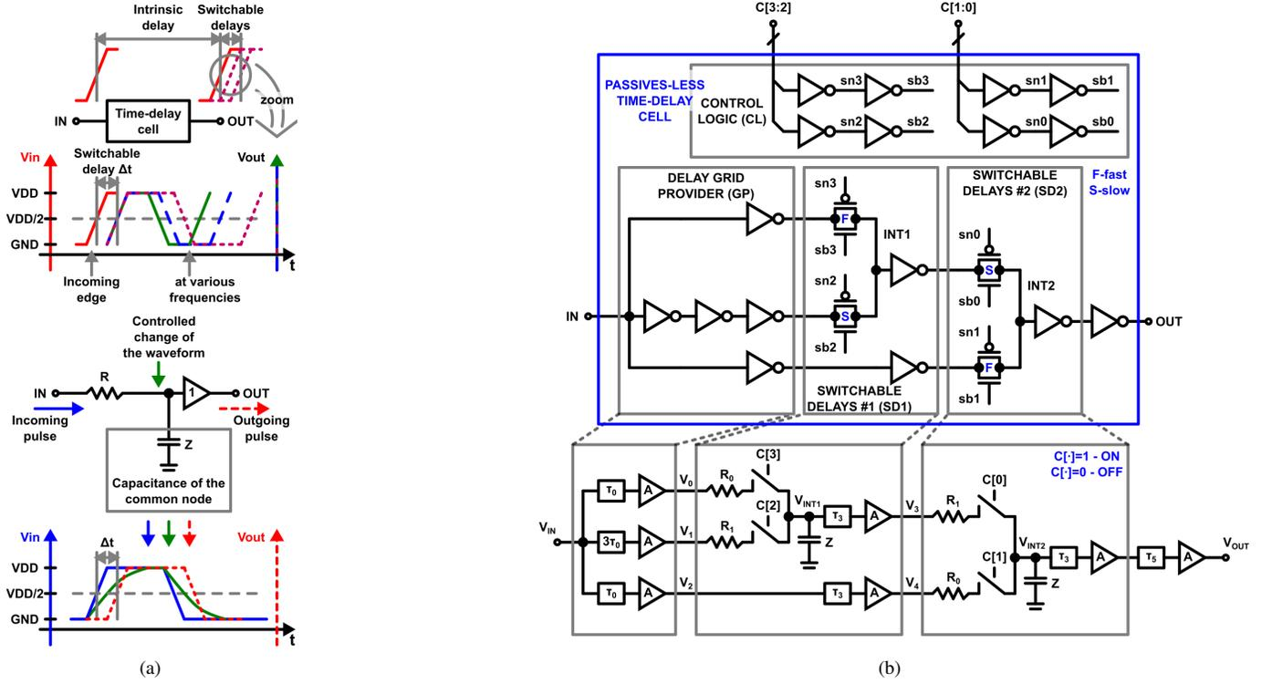
Fig. 2. (a) Definition of delays in this work and proposed delaying principle; (b) implemented delay cell schematic with its idealized model.
