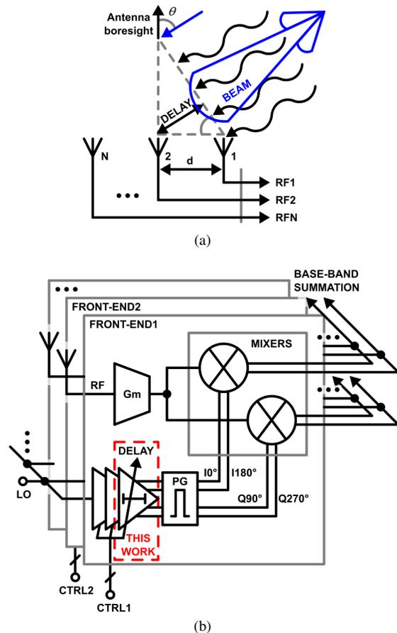
Fig. 1. (a) Concept of beamsteering; (b) conceptual diagram of the receiver.
