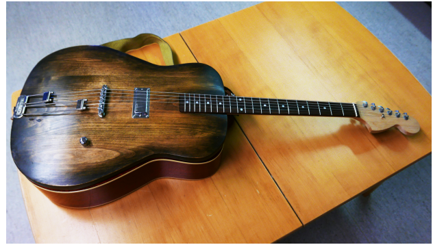
Figure 8. Electric guitar with an actuated body built by luthier Juhana Nyrhinen. Audio transducers have been mounted into the sound box, providing a guitar with an integrated amplifier/speaker.
