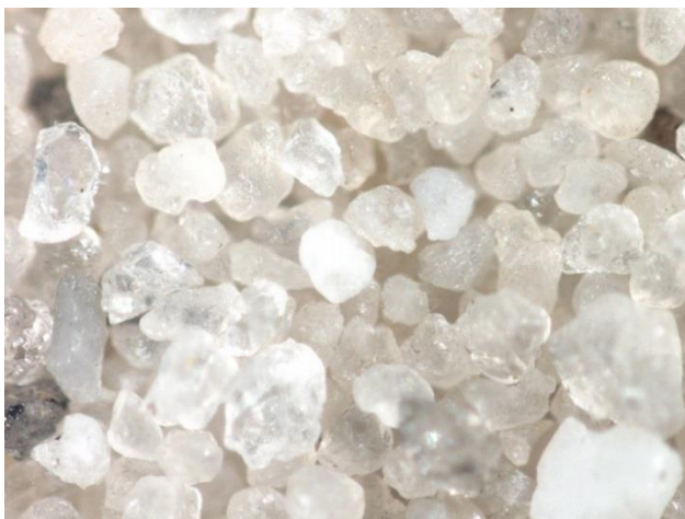
Fig. 4. Micrograph of foundry 4 sand reclaimed in 550 °C
