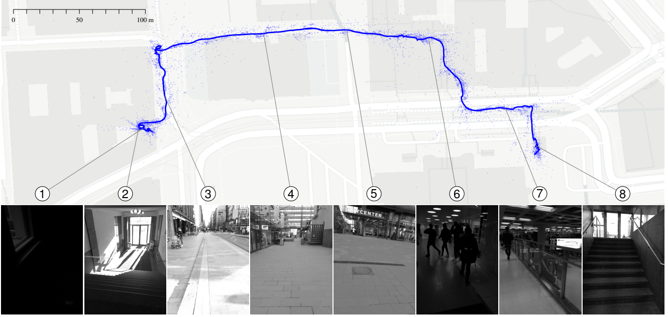
Figure 1: PIVO tracking on a smartphone (iPhone 6) starting from an office building (1–2), through city streets (3–5), a shopping mall (6), and underground transportation hub (7–8).
