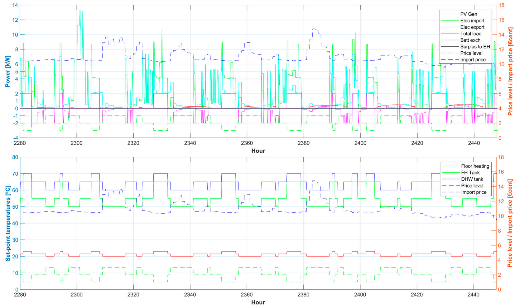
Figure 4. Example of the operation of the RBC from hours 2280 to 2448, corresponding to April 6 to 13 (Lowest LCC RBC parameters: Perc. PFP 12 h, Low: 20, High: 60). The top and bottom charts show the electricity and heat management actions, respectively. “Price level” is to be interpreted as Low = 1, Normal = 2, High = 3. Positive values of “Batt exch” indicate charging; negative values discharging.
