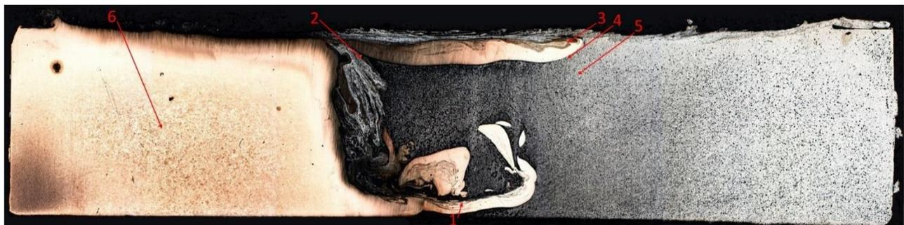
**Fig. 12** Optical macrograph of the optimized weld, areas of interest detailed by Fig. 13 are marked from 1 to 6
