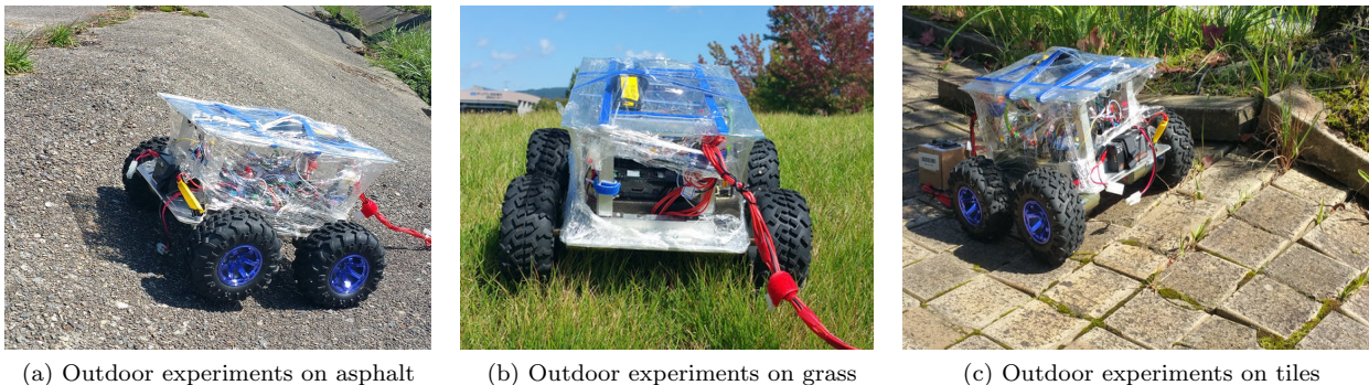
Figure 5: Rusti V2.0 with all-terrain wheels and external 3-axis accelerometer sensor for outdoor field experiments carried out on different terrains.
