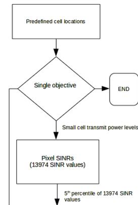
Fig. 1. Flow chart of transmit power optimization
