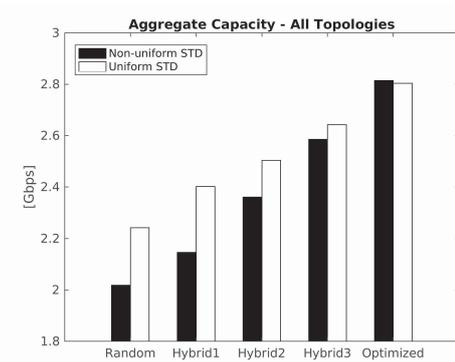
Fig. 11. Aggregate capacity performance comparison of all topologies
