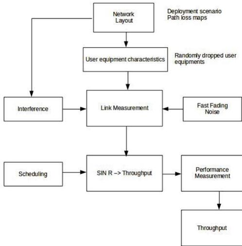
Fig. 4. System level simulator block diagram
