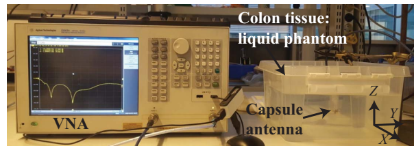
Fig. 6. Illustration of the in-vitro measurement setups.
