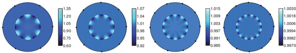
FIG. 2. Outputs of Algorithm 5.1 for  $N = 5, 7, 9, 11$  (recall that  $N + 1$  is the number of electrodes). The point-like electrodes are located at the polar angles  $\theta_j = 1^\circ + \frac{j}{N+1}360^\circ$ ,  $j = 0, 1, \dots, N$ . The values of  $\varepsilon$  used in the computations are 14, 12, 8 and 8, respectively.
