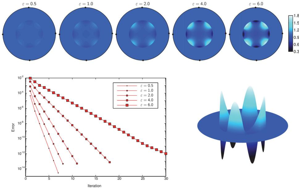
FIG. 1. Top row: Outputs  $\sigma^\varepsilon$  of Algorithm 5.1 with different values of the perturbation size parameter  $\varepsilon > 0$ . The point-like electrodes are located at the polar angles  $\theta = 1^\circ, 91^\circ, 181^\circ, 271^\circ$ . Bottom left: The discrepancy (6.1) between consecutive iterates of Algorithm 5.1. Bottom right: A surface plot of  $\sigma^\varepsilon$  corresponding to  $\varepsilon = 6.0$ .
