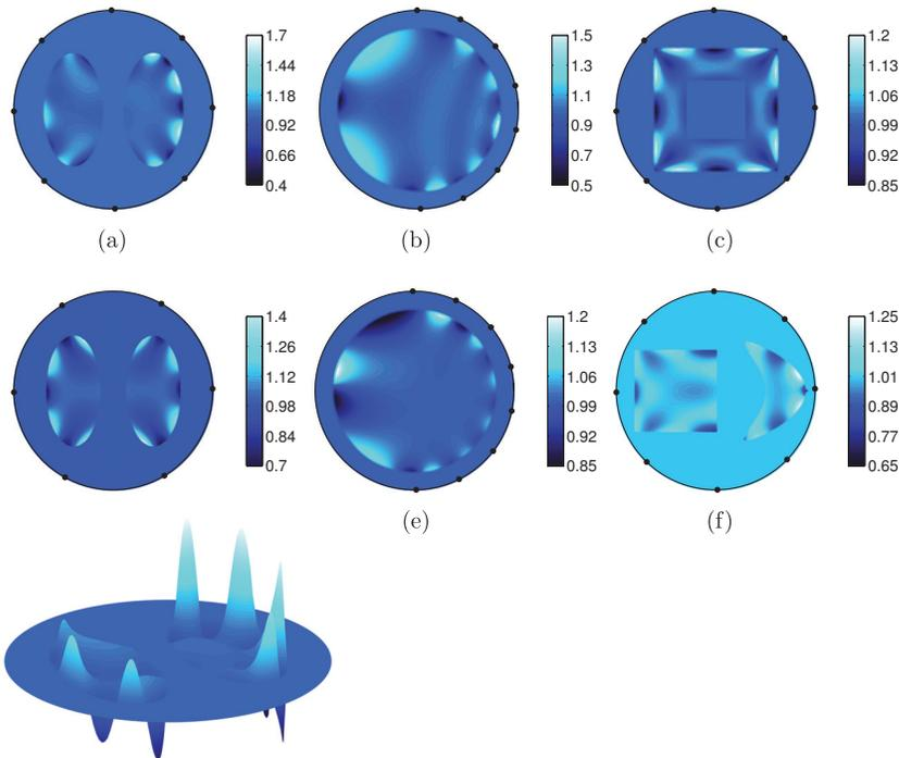
FIG. 3. (a)–(f) Perturbed conductivities produced by Algorithm 5.1 for the shown electrode configurations. Bottom left: A surface plot of the conductivity (a).
