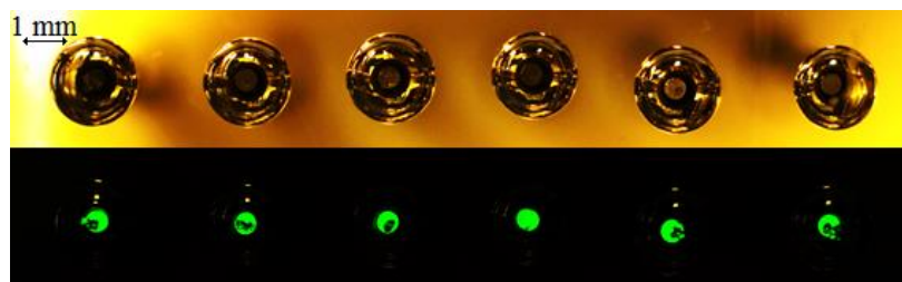
Figure 3- Photos of bubbles taken from a single measurement cycle: a typical picture from the needle array taken for automated bubble size measurement (top), and a second picture from the same bubble array aided by optical fiber backlighting for automated particle detection (bottom)
