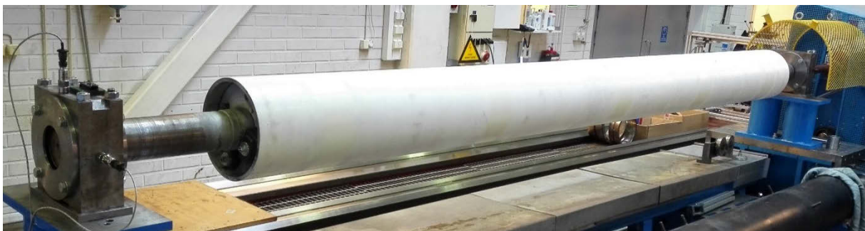
Figure 2 Test rotor and the measurement setup in the tending side bearing housing.
