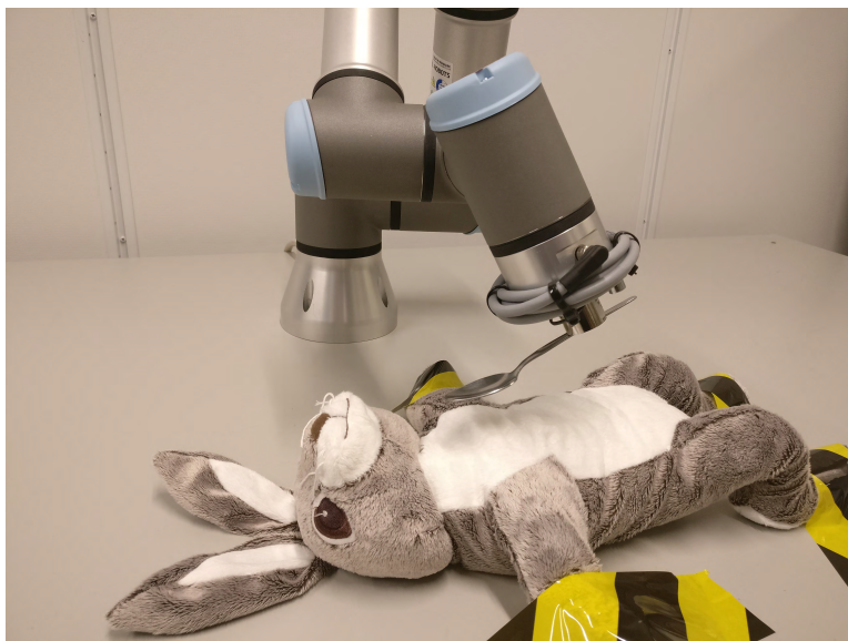
FIGURE 1. A robotic arm was used to move a set of instruments to simulate a remote surgery of a dummy patient.
