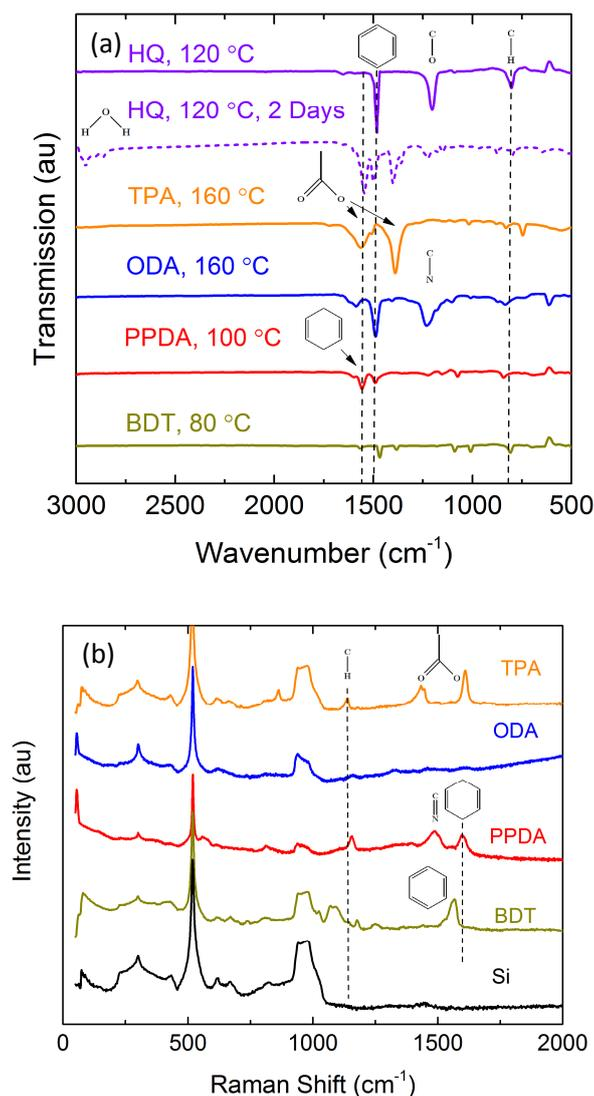
**Fig. 5** (a) FTIR and (b) Raman spectra for representative hybrid films deposited with  $\text{Cu}(\text{dmap})_2$  and the different organic precursors; the FTIR spectra are transmission spectra after subtraction of the Si spectrum.
