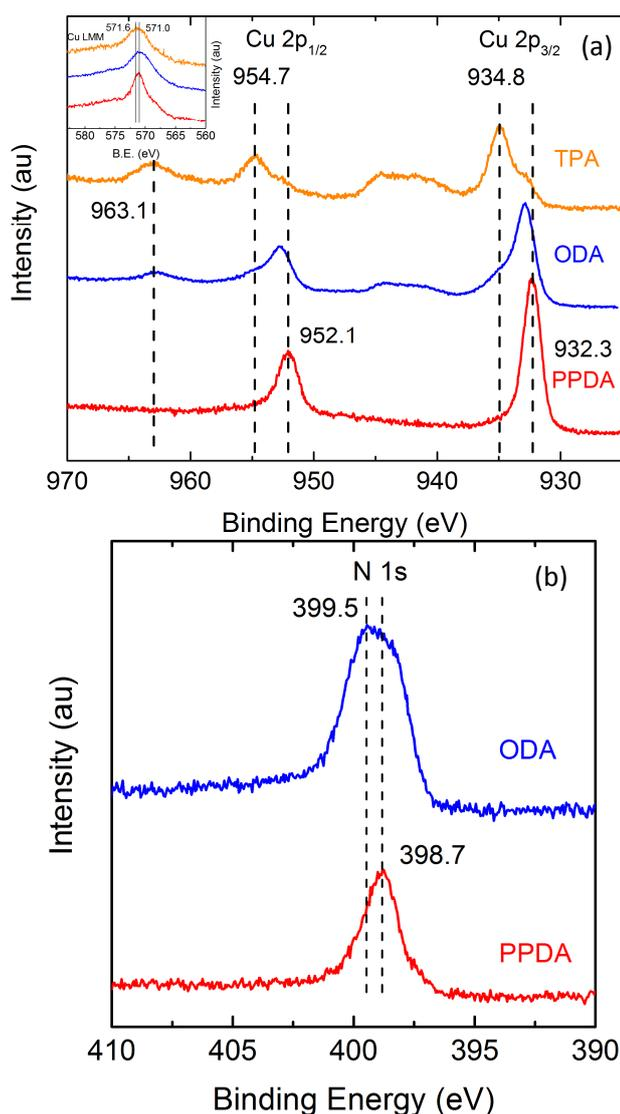
**Fig. 6** XPS spectra of Cu-organic films deposited with  $\text{Cu}(\text{dmap})_2$ : (a) Cu 2p region of Cu-TPA, Cu-ODA and Cu-PPDA, the insert shows the Cu LMM Auger peak, (b) N 1s region of Cu-ODA and Cu-PPDA.
