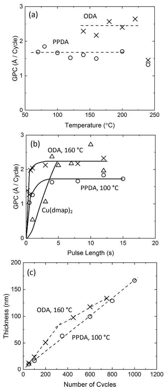
**Fig. 2** Optimization of the  $\text{Cu}(\text{dmap})_2$ +ODA (o) and  $\text{Cu}(\text{dmap})_2$ +PPDA (x) process parameters on Si: (a) GPC versus deposition temperature; (b) GPC versus precursor pulse lengths, triangles are for the  $\text{Cu}(\text{dmap})_2$  pulse; (c) film thickness versus number of ALD/MLD cycles. In (b) and (c), the deposition temperature was 160 °C for the  $\text{Cu}(\text{dmap})_2$ +ODA process, and 100 °C for the  $\text{Cu}(\text{dmap})_2$ +PPDA process.
