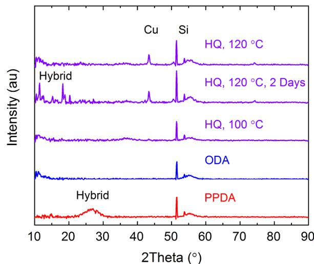
**Fig. 3** Representative GIXRD patterns for films deposited with the  $\text{Cu}(\text{dmap})_2$  and PPDA (100 °C, 1000 cycles) or ODA (160 °C, 750 cycles), and patterns for two films deposited with HQ at 120 °C: as-deposited and air-stored for 2 days.
