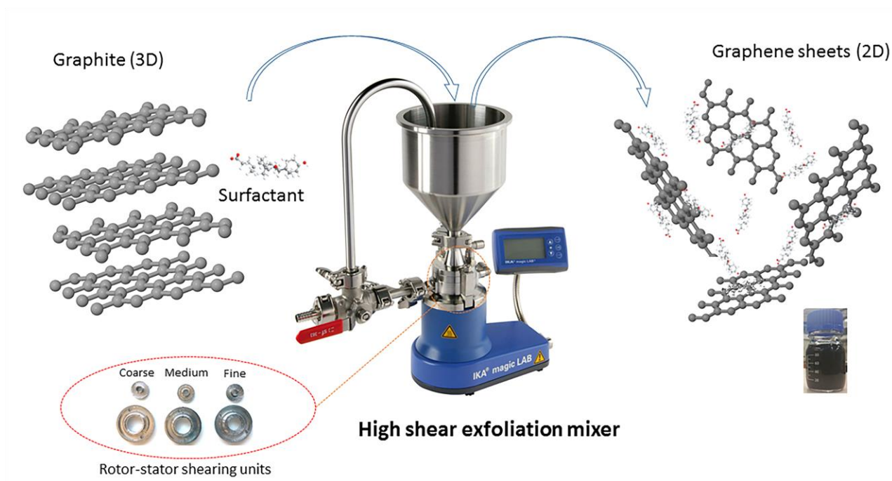
Figure 1. Schematic illustration of the exfoliation process using a high shear colloidal mixer. The starting graphite was first added to PVP or SC solution and subjected to high shear mixing. The resulting mixture was then centrifuged to remove unexfoliated graphite.
